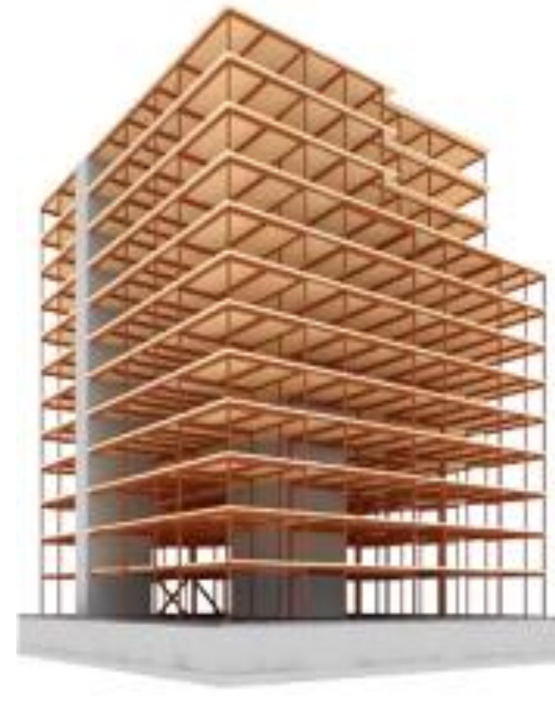
Steel Frame + MT Floors Hybrid 9 - 15 bf/sq.ft.
